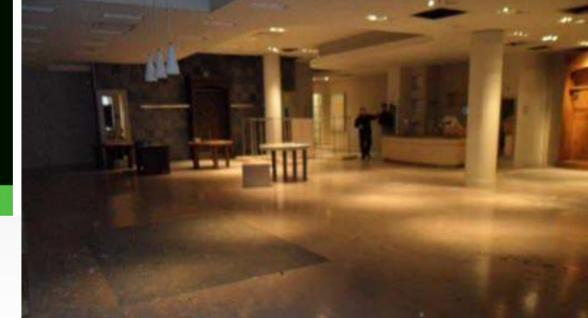
Visible columns before renovations. Columns will be removed and replaced with new beams around the perimeter to distribute the weight of the floor above.
