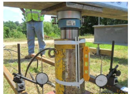
*Movement and fluctuations of the steel pile are measured and recorded.*
