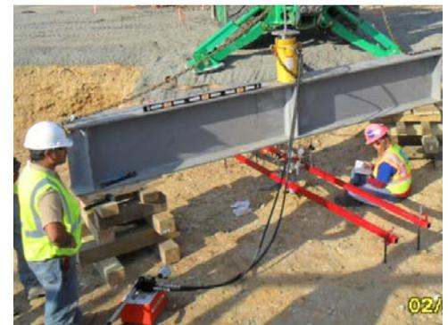
*The helical pile is at the center of this field test beneath the horizontal beam. A hydraulic jack is used to provide pressure on the pile.*
